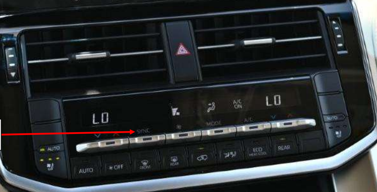
FRONT AUTO AC WITH 4-ZONE INDEPENDENT CONTROL
